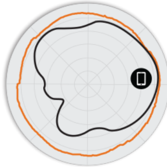
Figure 3. T610o 5GHz Azimuth Antenna Patterns
