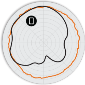
Figure 2. T610o 2.4GHz Azimuth Antenna Patterns
